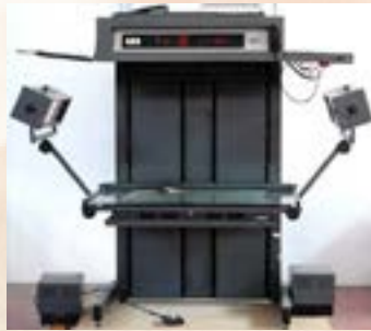
REPRO CAMERA: Was used to shoot composed pages, and produce films (Below), for plate making.
