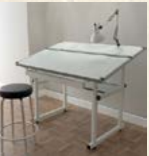
DRAUGHTING TABLE : Used by paste-up artistes. . Rules were manually drawn using rotaring® pens, and blocks or columns of text were pasted in position using cow Gum (below).
